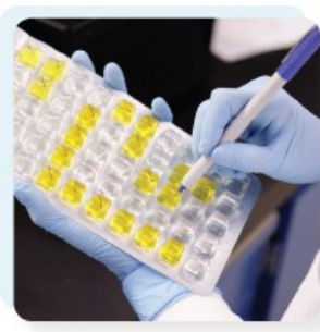
Fig 4 (below): Checking for positive bacterial results using the MPN method (Photo by IDEXX).
