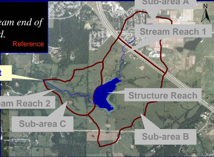
The map shows a watershed boundary in red. A blue stream flows from the top right towards the bottom left. A blue reservoir is located in the center. The watershed is divided into three sub-areas: Sub-area A (top right), Sub-area B (bottom right), and Sub-area C (bottom left). Stream Reach 1 is the upper portion of the stream, Stream Reach 2 is the lower portion, and Structure Reach is the area around the reservoir. A north arrow is in the top right corner.
